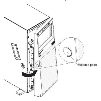
3. Disengage the hinge assembly form the chassis to release the bezel out of the chassis.
