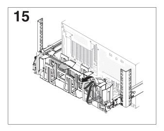
Secure the cable management arm if you are shipping the server in a rack.
