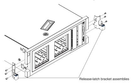
b. Secure the bracket with three M3.5 screws that come with this kit.
