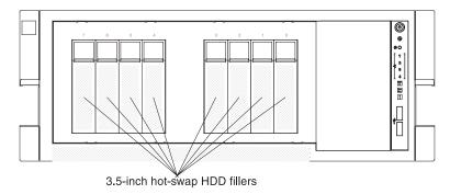
c. Install the 3.5-inch simple-swap HDD fillers if necessary.
