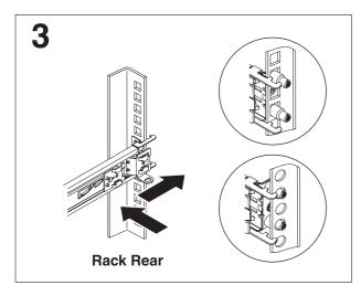
Install the rear end of the slide rails.
