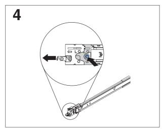
Install the front end of the slide rails.
