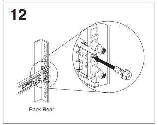
Secure the cable management arm and the server in the rack for shipping if needed.
