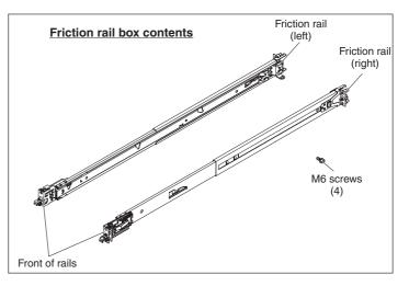
**Note:** If the slide rails in your rack installation kit came with shipping thumbscrews, remove them before you begin the following installation procedure.
