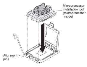
b. Twist the handle on the microprocessor tool counterclockwise to insert the microprocessor into the socket.
