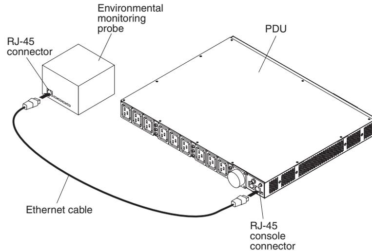
3. Make sure that the PDU has a network connection, the power cord is connected, and the power to the PDU is turned on. The environmental monitoring probe is automatically recognized by the PDU.
