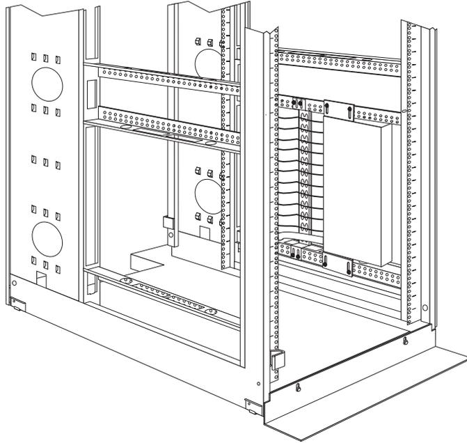
**Note:** To route a power cord through the cable-management bracket, route the cord through an opening in the bracket and against an upper or lower tab on the bracket, as shown in the following illustration. Use cable straps as required.
