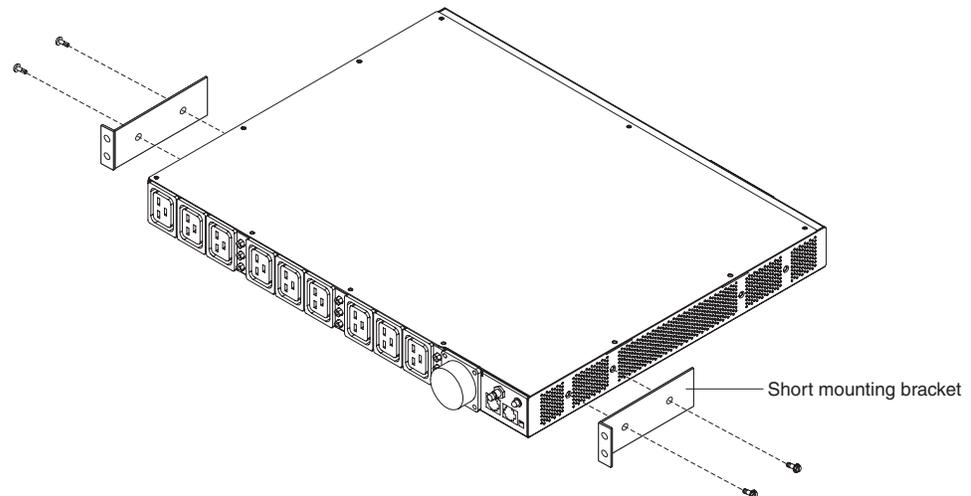
2. Attach the brackets to the PDU with two M3 x 5 screws per bracket. Use the screws that come with the PDU.
