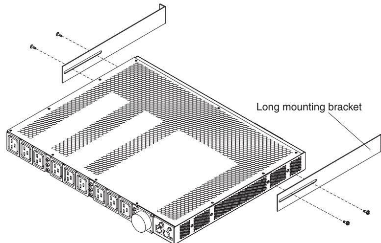
3. Orient the PDU so that the vent holes are facing up. Hold the PDU at a slight angle and carefully insert it into the 1U mounting space in the rack cabinet. Pushing in slightly on both of the long mounting brackets helps clear the brackets from the rack flanges.
