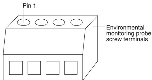
**Note:** External contact device 1 is connected between pins 1 and 2. Device 2 is connected between pins 3 and 4 (as labeled to show device 1 and 2). External contact devices can be normally open or normally closed.
