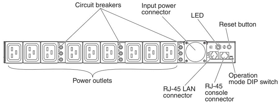
The following illustration shows the components and controls on the front of the non-monitored PDU models.
