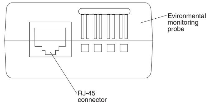
The environmental monitoring probe kit comes with one environmental monitoring probe, screws, hook-and-loop fasteners, tie wrap, and cable. You can install the device anywhere you want on the rack. To attach the environmental monitoring probe, use either the hook-and-loop fasteners or mount the probe on the screw (the environmental monitoring probe has a universal slot on the back that makes it mount easily on the screw and in any direction).
