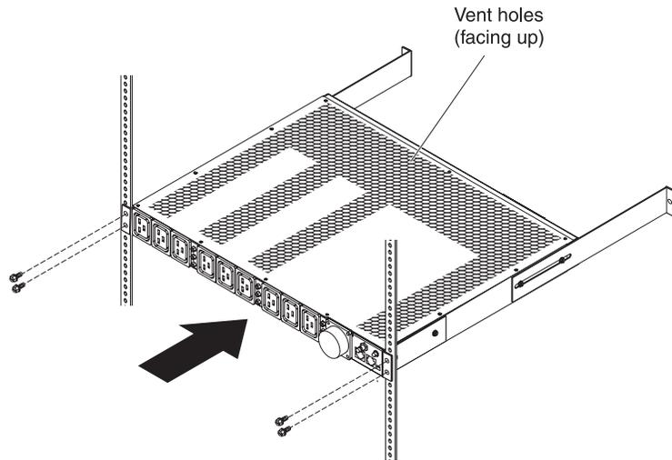
5. Secure the long mounting brackets and the 1U blank filler panel to the rack cabinet.
