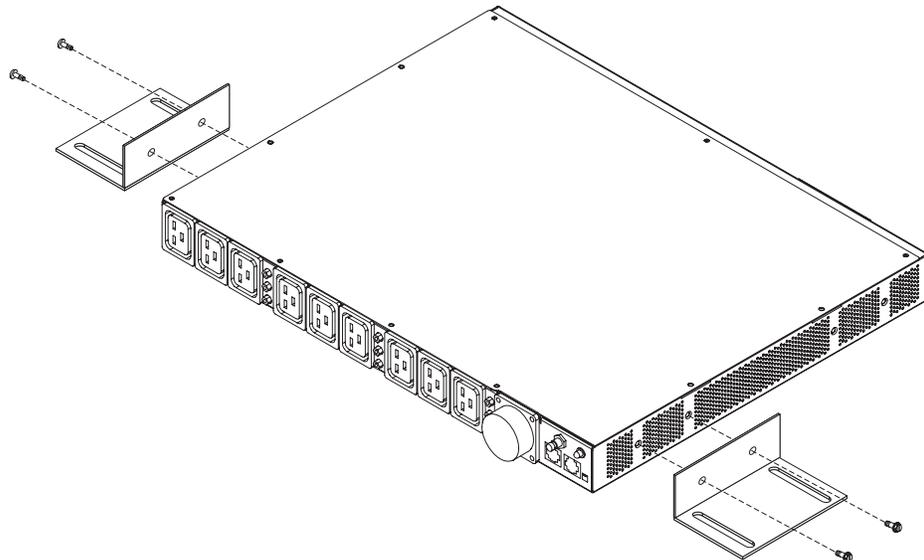
2. Hold the PDU in the side of the rack cabinet, and attach the vertical mounting brackets to the side braces with four M6 screws and nuts that come with the PDU.
