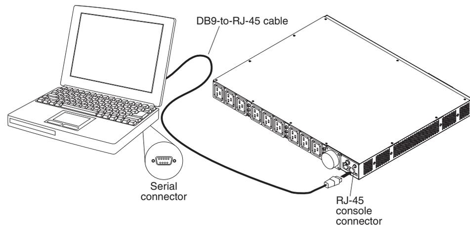
If your workstation or notebook computer does not have a DB-9 serial connector, you can use a DB-9-to-USB converter cable to connect the PDU to a workstation or notebook computer.
