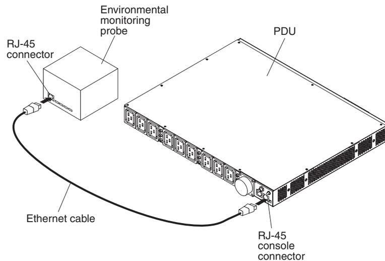
For more information about the environmental monitoring probe, see Chapter 6, “Using the environmental monitoring probe,” on page 49.
