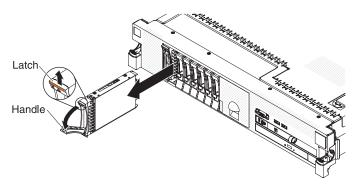
**Attention:** To maintain proper system cooling, do not operate the server for more than 10 minutes without either a drive or a filler panel installed in each bay.
