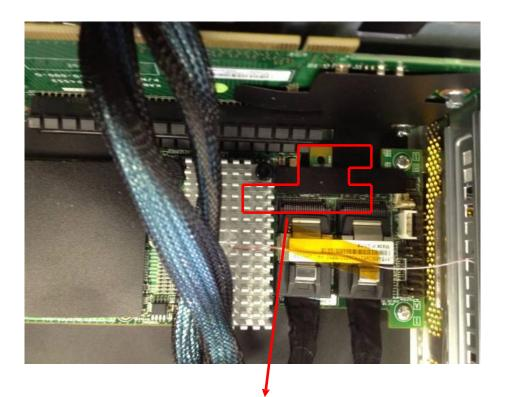
Use the screw for alignment support, note upper part should be folded to another side to fit properly.
