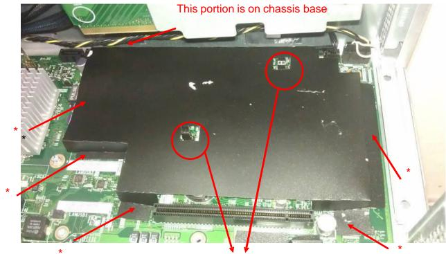
Use the stand out connectors to position the Mylar.
