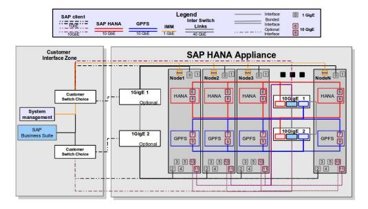
**Note:** The "Customer Switch Choice" labeled switches are either 1 Gigabit Ethernet adapter or 10GbE SFP+ switches provided by you or IBM. Make the switch uplink redundant when possible.
