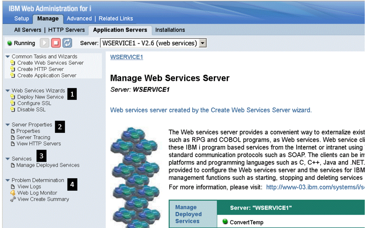
Figure 23: Manage server panel
