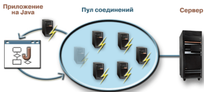
Figure 3: Java program getting a connection from an AS400ConnectionPool to a server
