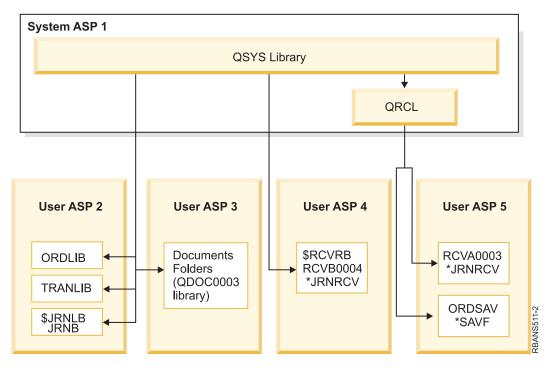
Figure 7. User ASP configuration after reclaiming storage
