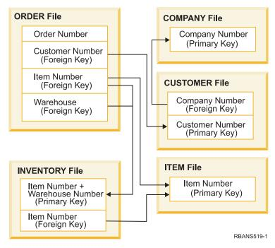
Figure 25. Restoring a referential constraint network
