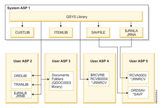
Figure 5. User ASP configuration before failure
