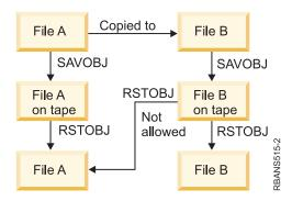
Figure 21. Restoring a copy of a file
