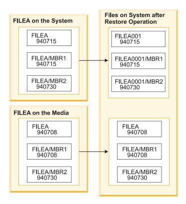
Figure 22. Restoring database files with different creation dates
