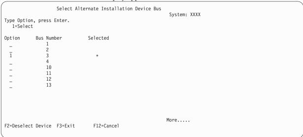
Type 3, and press Enter. This will verify the address of an alternate installation device attached to the system and determine whether it is enabled or disabled.
