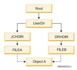
Figure 26. An object with hard links-Example
