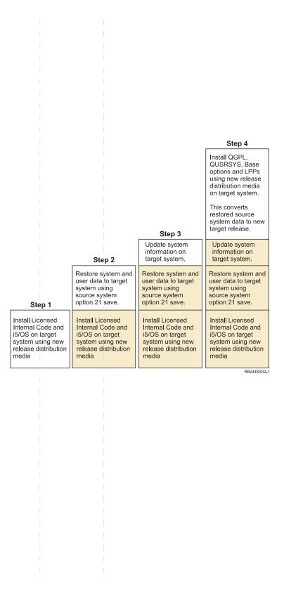
Figure 32. Recovery steps for restoring previous release user data to a new system
