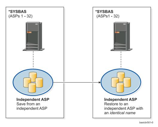
Figure 15. Save data from an independent ASP and restore it to an independent ASP with an identical name
