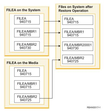
Figure 23. Restoring database files with different creation dates
