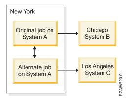
Telnet establishes a session from New York to Chicago. You also want to go to the Los Angeles system and remain connected to the Chicago system. You can start an alternate job on the New York system, using System Request option 11. Use the Telnet command to establish a session to the Los Angeles system. You can get to another system (Houston, for example) by starting another Telnet session from the Chicago system or the Los Angeles system.
