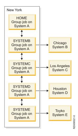
System A in New York contains Home Group job on System A, with bidirectional arrows down a chain connecting to, in order: System B group job on System A, System C group job on System A, System D group job on System A, and System E group job on System A. Each System group job on A has an arrow pointing to the correlating remote system (B, C, D, and E).
