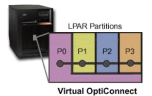
Virtual OptiConnect emulates external OptiConnect hardware by providing a virtual bus between logical partitions. You can use virtual OptiConnect without any additional hardware requirements. To use virtual OptiConnect, you only need to purchase OptiConnect for i5/OS (a priced optional feature).
