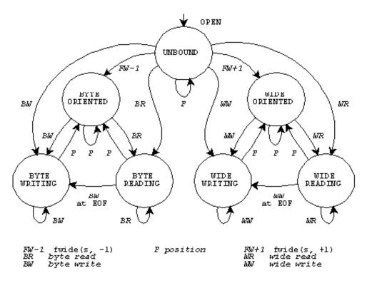
Each of the circles denotes a stable state. Each of the lines denotes a transition that can occur as the result of a function call that operates on the stream. Five groups of functions can cause state transitions.
