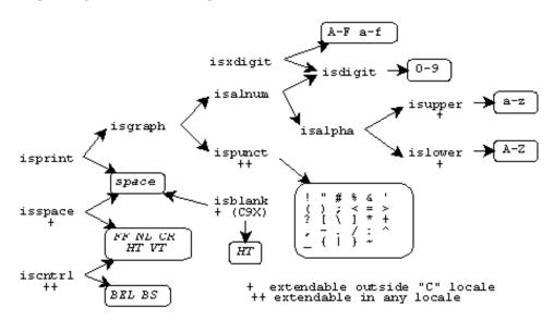
The diagram tells you that the function isprint (page 58) returns nonzero for *space* or for any character for which the function isgraph (page 57) returns nonzero. The function isgraph, in turn, returns nonzero for any character for which either the function isalnum or the function ispunct returns nonzero. The function isdigit, on the other hand, returns nonzero only for the digits 0-9.
