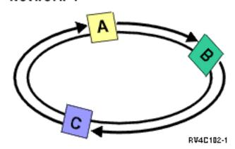
With the default (or normal) settings, a heartbeat message is sent every 3 seconds from every node in the I cluster to its upstream neighbor. For example, if you configure Node A, Node B, and Node C on Network 1, Node A sends a message to Node B, Node B sends a message to Node C, and Node C sends a message I to Node A. Node A expects an acknowledgment to the heartbeat from Node B as well as an incoming
