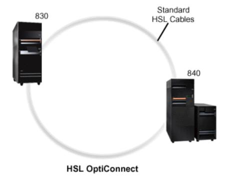
High-speed link (HSL) OptiConnect provides high speed system-to-system communication for PCI-based models. It requires standard HSL cables, but no additional hardware is required. To use HSL OptiConnect, you need to purchase OptiConnect for i5/OS software (a priced optional feature). The OptiConnect software will choose the Virtual OptiConnect path over a HSL or SPD OptiConnect external path if multiple paths are available.
