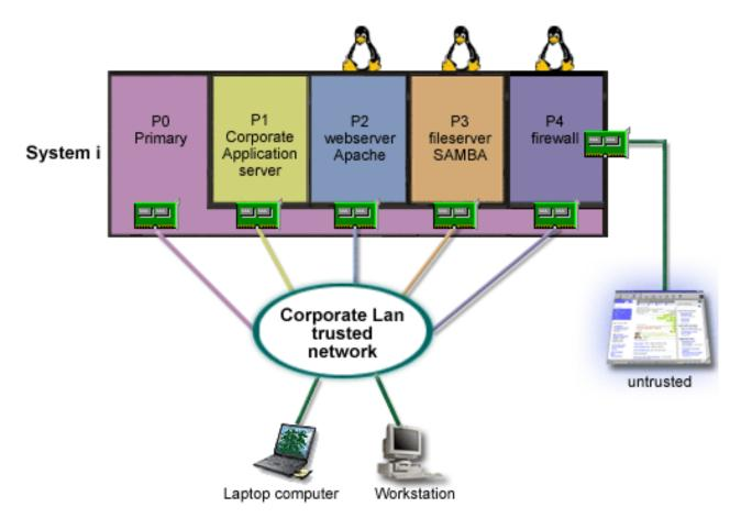
You had the hardware resources on your server to create another guest partition using System i Navigator. You installed Linux in partition P4. The firewall is built into the kernel that you are using. Your Linux firewall partition owns a directly-attached LAN adapter that protects the entire system from untrusted data.
