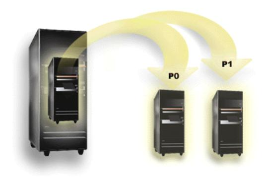
Logical partitioning is the ability to make a system run as if it were two or more independent systems. Each logical partition operates as an independent logical server. However, each partition shares a few physical system attributes such as the system serial number, system model, and processor feature code. All other system attributes may vary among partitions.
