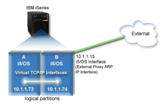
In this example, TCP/IP traffic from partition A runs across the virtual Ethernet to the 10.1.1.74 interface on partition B. Because10.1.1.74 is associated with the external proxy ARP interface 10.1.1.15, the packets continue out of the virtual Ethernet using the proxy ARP interface.
