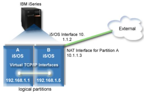
In this example, any existing TCP/IP traffic for the server runs over the 10.1.1.2 interface. A new
