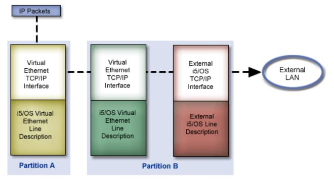
IP traffic initiated by Partition A goes from its virtual Ethernet interface to the virtual Ethernet interface on Partition B. By implementing any one of the three TCP/IP techniques described below, you can enable the IP packets to continue on to the external interface and toward their destination.
