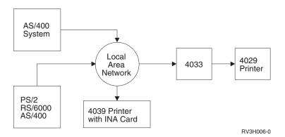
Figure 1. Physical view of ASCII LAN-attached printers
