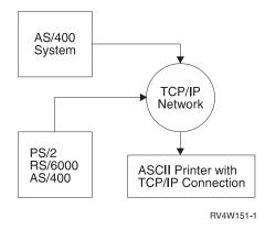
Figure 3. Physical view of ASCII TCP/IP network-attached printers
