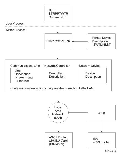
Figure 2. Software view of ASCII LAN-attached printers
