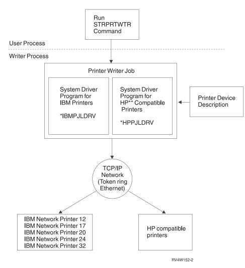
Figure 4. Software view of ASCII TCP/IP network-attached printers using PJL
