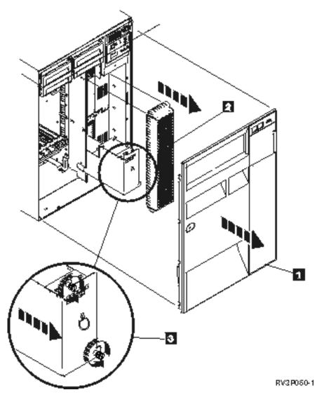
Figure 1. Removal of the battery power unit on Models 5xx, and expansion units FC 507x and FC 508x.
