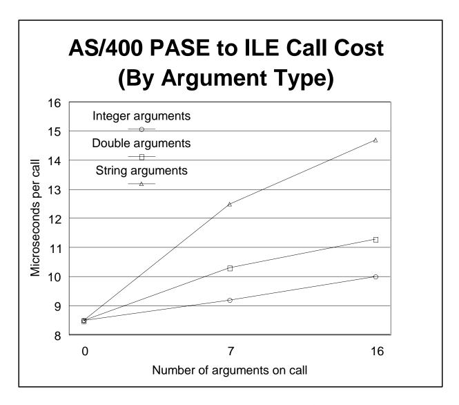
Figure 21.2 Cross environment calls comparing iSeries PASE to ILE and ILE to ILE
