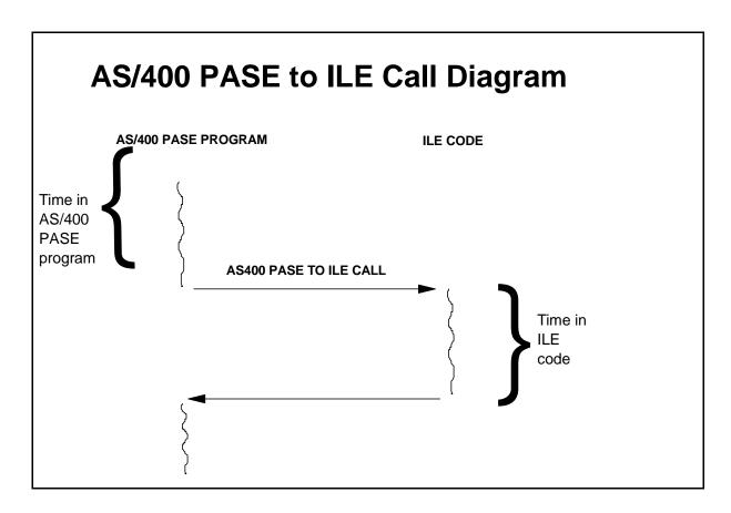
Figure 21.3 iSeries PASE to ILE Call Flow
