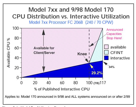
Figure 2.4. Model 7xx Utilization Example
