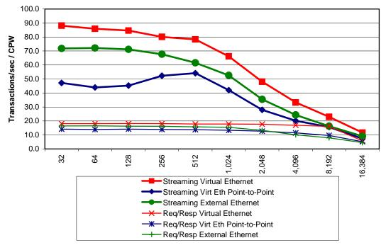
Netperf consists of C programs which use a socket connection to read and write data between buffers. The CPW results don't attempt to factor out the minimal application CPU requirements. Thus, the CPU results include the primitive Netperf application, socket, TCP, and ethernet operation costs. A real user application will only have this type of processing as a percentage of the overall workload.
