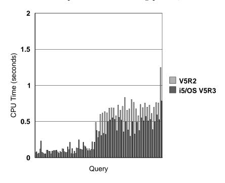
Figure 4.3 Runtime comparison for queries in the 2 seconds to 200 seconds range
