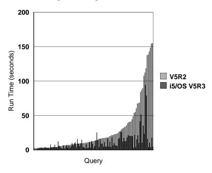
Figure 4.4 CPU time comparison for queries in the 2 seconds to 200 seconds range
