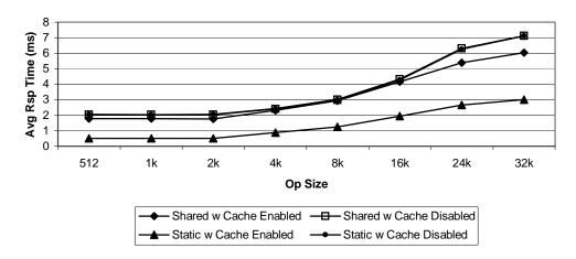
(The performance characteristics of Static and Dynamic disks are identical) As shown above, there may be only a subtle difference in average response time between Shared with cache enabled or disabled, so it is probably not worth enabling the cache for Shared disks. However, the difference will become more pronounced as the storage subsystem becomes busier.
