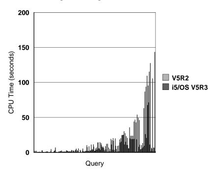
Figure 4.5 Runtime comparison for long running queries (400 seconds to 5500 seconds)
