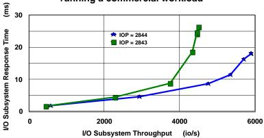
32 ESS F20 LUNs attached via 2 2766 (1Gb) IOAs and 2 IOPs 100% ESS read cache hits
