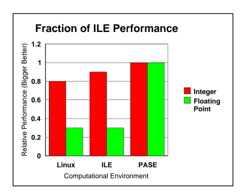
One virtue of the i870, i890, and i825 machines is that the hardware floating point unit can make up for some of the code generation deficit due to its superior hardware scheduling capabilities.
