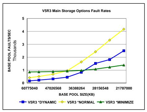
Figure 11.4 V5R3 Main Storage Options on a Power4 System - Page Fault Rates
