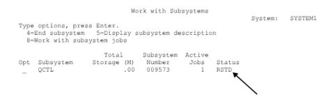
Figure 3. WRKSBS display with controlling subsystem in restricted state
