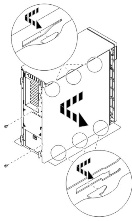
Figure 1. Remove system unit side cover
