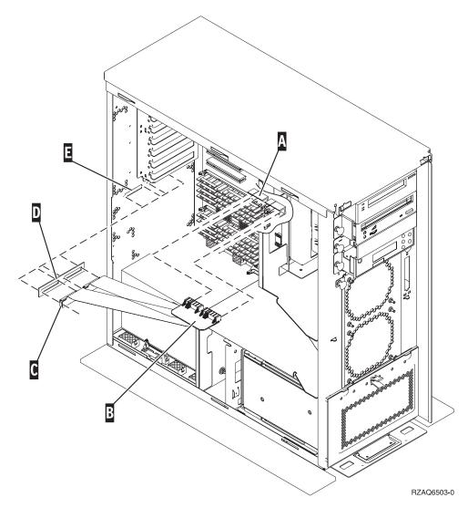
Figure 2. Installing the 7002 internal flex cable
