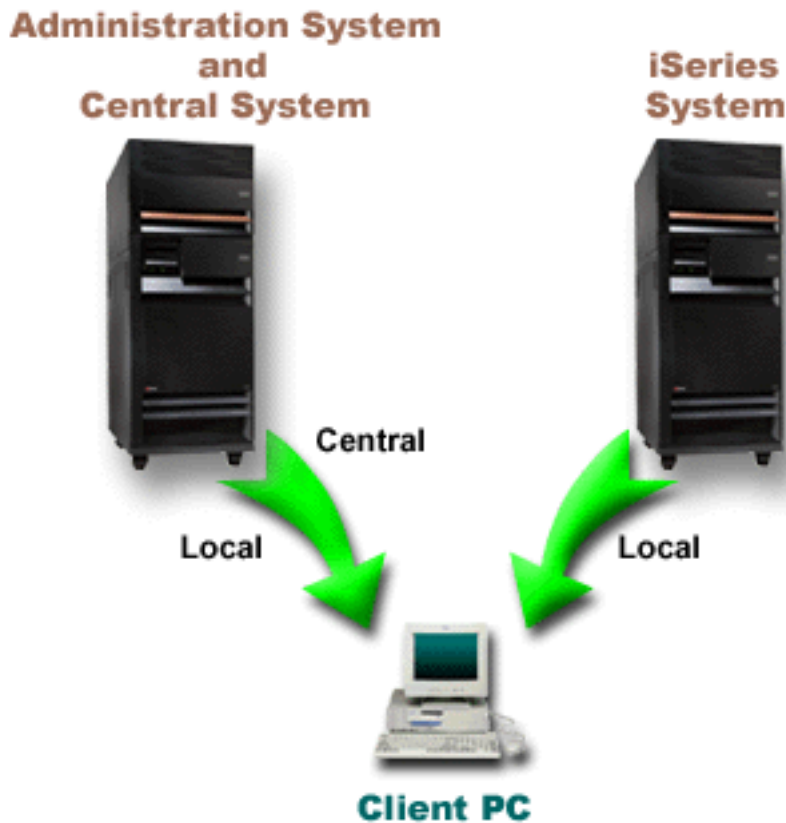
Figure 3. The administration system and the central system can be the same system. It does not change the function of Application Administration or Management Central. When a Client PC connects to a system, the Local Settings come from the system that you connect to. When you connect to an administration system, the Central Settings are sent to your Client PC from the administration system.
