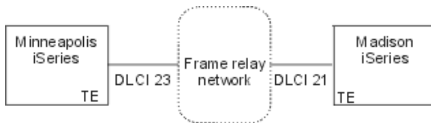
Figure 8. SNA Direct Connection between Minneapolis and Madison Systems
