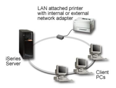
Although the hardware support for printing through a remote output queue using LPR/LPD is extensive, not all printers will support it. You should verify that the printer you would like to use supports this printing method. The IBM Knowledge Base document 17690939 "Support for Various ASCII Printers" maintains a list of protocols supported by common printers.
