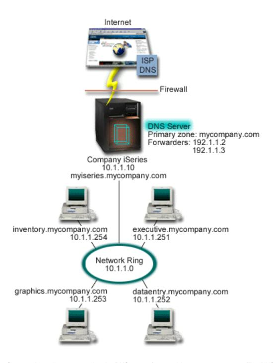
Suppose host dataentry queries the DNS server for "graphics.mycompany.com". The DNS server will use its own zone data and respond with the IP address 10.1.1.253.
