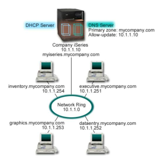
Previous versions of DHCP and DNS were independent of each other. If DHCP assigned a new IP address to a client, the DNS records had to be manually updated by the administrator. In this example, if the graphics file server's IP address changed because it is assigned by DHCP, then its dependent clients would be unable to map a network drive to its host name because the DNS records would contains the file server's previous IP address.
