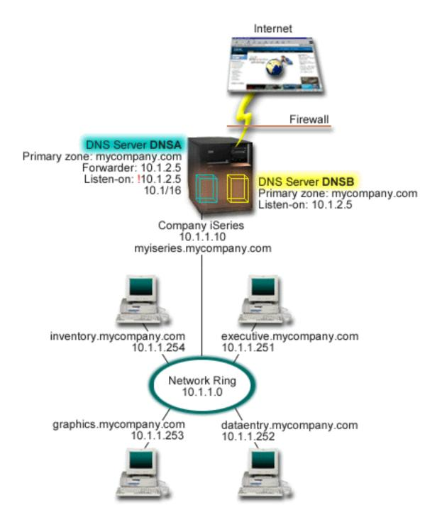
The external server, DNSB, is configured with a primary zone mycompany.com. This zone data includes only the resource records that are intended to be part of the public domain. The internal server, DNSA, is configured with a primary zone mycompany.com, but the zone data defined on DNSA contains intranet resource records. The forwarders option is defined as 10.1.2.5. This will force DNSA to forward queries it cannot resolve to the DNSB server.
