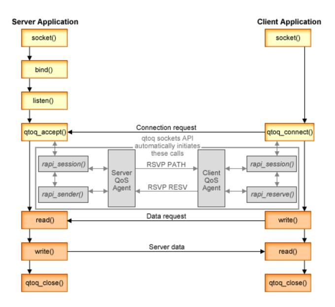
**qtoq flow of events:** The following sequence of socket calls provide a description of the graphic. It also describes the relationship between the server and client application in a connection-oriented design. These are modifications of the basic Sockets APIs.
