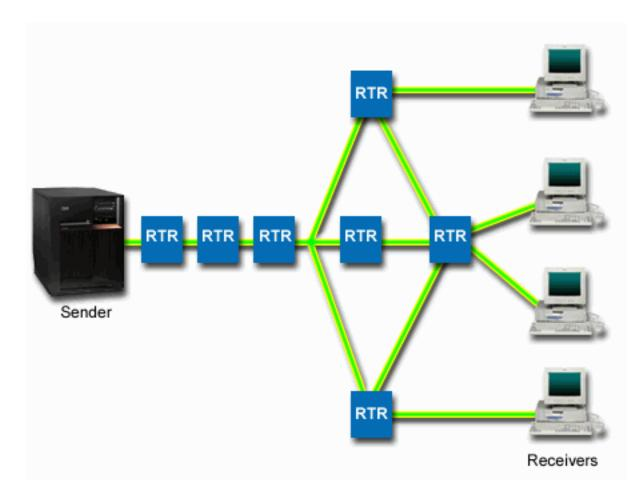
The RSVP-enabled application on the server detects a connection request from the client. In response, the server's application issues a PATH command to the client. This command is issued using the RAPI APIs or qtoq QoS sockets APIs and contains router IP address information. A PATH command contains information about the available resources on the server and the routers along the path, as well as, route information
