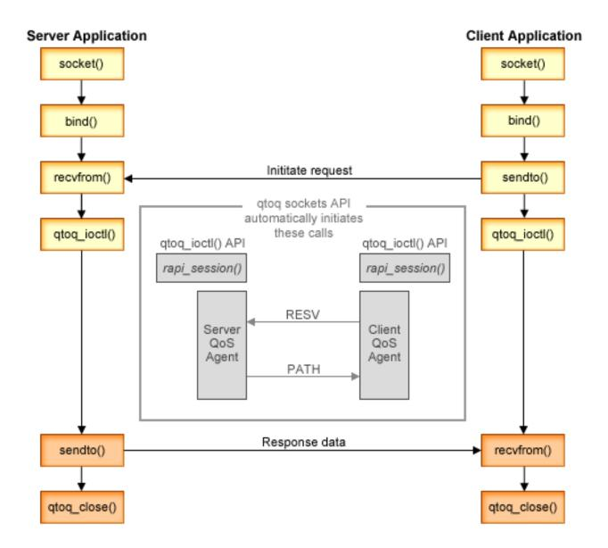
**qtoq flow of events**: The following sequence of socket calls provide a description of the graphic. It also describes the relationship between the server and client application in a connectionless design. These are modifications of the basic Sockets APIs.
