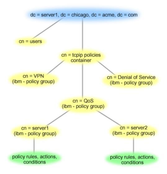
Server1 at the top (dc=server1,dc=chicago,dc=acme,dc=com) is the server on which the directory server resides. The other servers, such as cn=QoS or cn=tcpip policies are where the QoS servers reside. So on cn=server1 the default DN would read cn=server1,cn=QoS,cn=tcpip
