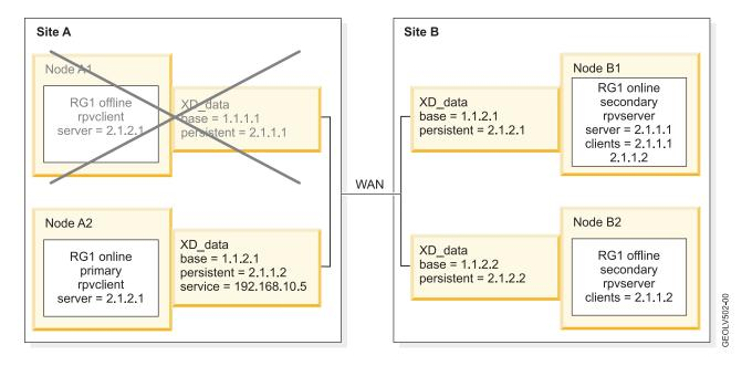
The following figure shows the GLVM configuration after the resource group falls over to the other site and remains active there. At this point, the failed nodes at the failed site have rejoined the cluster.
