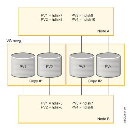
This configuration eliminates most potential single points of failure. However, a disaster can wipe out the entire cluster along with all copies of mission critical data.
