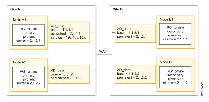
In the initial configuration of the GLVM cluster, the RPVclient for node A1 is bound to the persistent IP address 2.1.1.1 and uses the RPVserver on node B1, which is bound to persistent IP address 2.1.2.1. The corresponding setup is true for nodes A2 and B2 where the RPVclient on node A2 uses the RPVserver on node B2.
