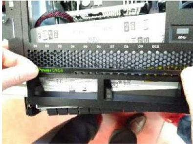
Figure 11. Assembling the front cover.
