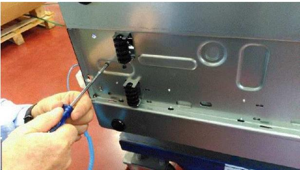
Figure 3. Removing pedestal screws.
