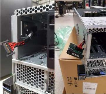
Figure 8. Control Panel Cable.
