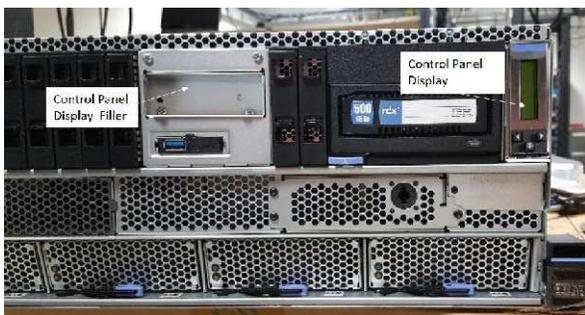
Figure 7. Control Panel Display in a standalone system.
