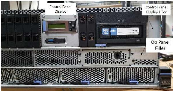
Figure 6. Control Panel Display in a racked system.
