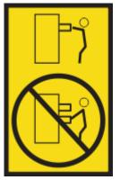
• (For fixed drawers.) This drawer is a fixed drawer and must not be moved for servicing unless specified by the manufacturer. Attempting to move the drawer partially or completely out of the rack might cause the rack to become unstable or cause the drawer to fall out of the rack. (R001 part 2 of 2)
