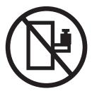
DANGER: Rack-mounted devices are not to be used as shelves or work spaces. Do not place objects on top of rack-mounted devices. In addition, do not lean on rack-mounted devices and do not use them to stabilize your body position (for example, when working from a ladder). (L002)
