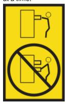
• (For fixed drawers.) This drawer is a fixed drawer and must not be moved for servicing unless specified by the manufacturer. Attempting to move the drawer partially or completely out of the rack might cause the rack to become unstable or cause the drawer to fall out of the rack. (R001 part 2 of 2)
