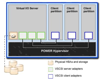
**Note:** The VIOS must be fully operational for the client logical partitions to be able to access virtual devices.
