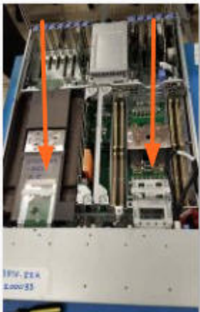
Figure 25. Replacing the air baffle
