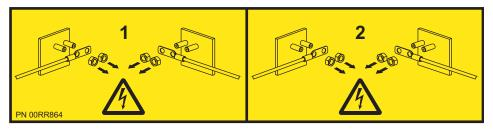
DANGER: Multiple power cords. The product might be equipped with multiple AC power cords or multiple DC power cables. To remove all hazardous voltages, disconnect all power cords and power cables. (L003)
