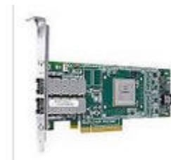
Figure 29. Qlogic QLE26920P Dual-port 16 Gb Fibre Channel adapter PCIe3 x8 LP Adapter
