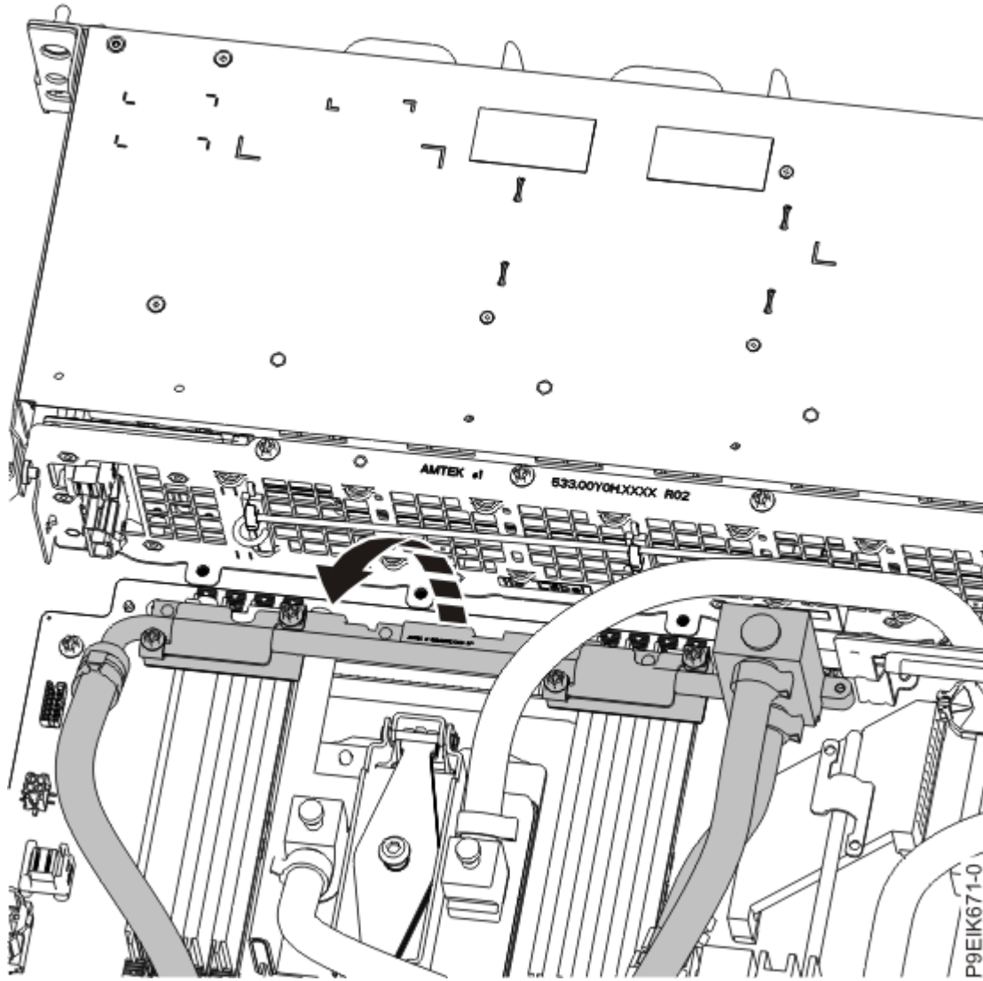
Figure 67. Moving the front pipe away
