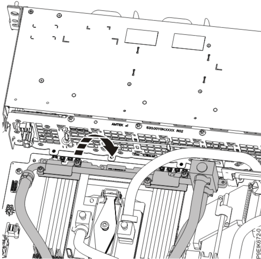
Figure 73. Replacing the front pipe and holder
