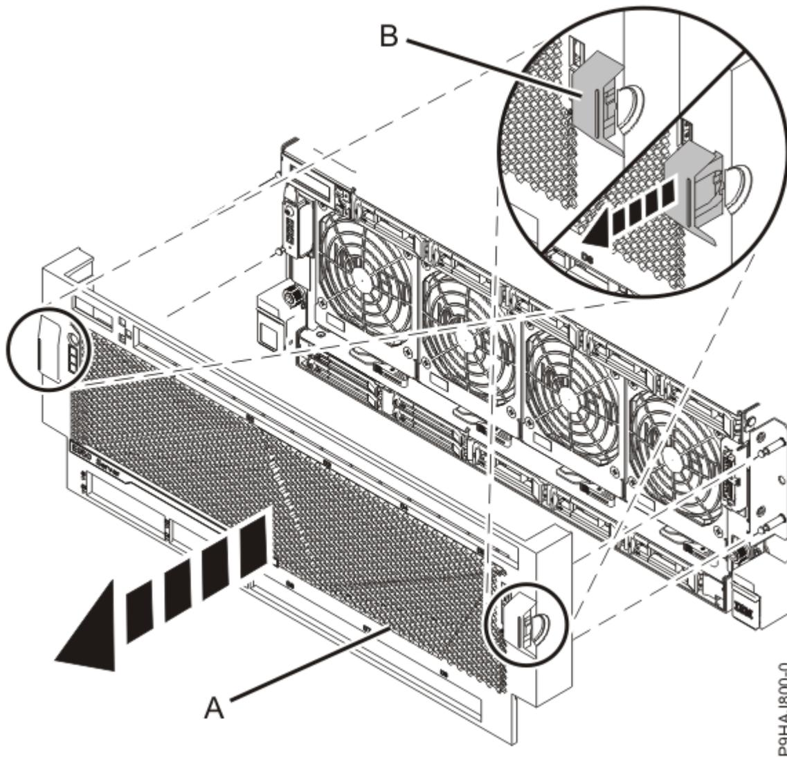
Figura 1: Removendo a Tampa Frontal
