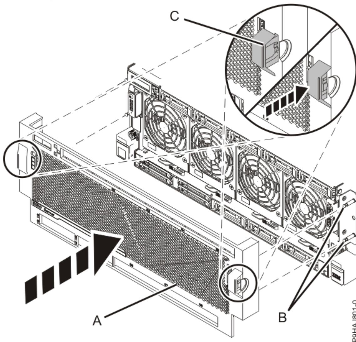
*Figura 6: Instalando a tampa frontal*
