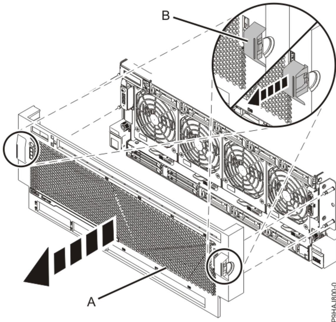
*Figura 2. Removendo a Tampa Frontal*
