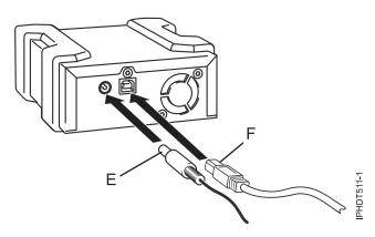
Figure 2. Rear view and connectors on the external drive
