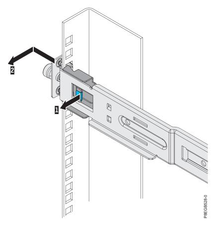
**8**. Remove the front bracket of the outer slide-rail from the rack by pulling the blue tab out 1 while you pull the end of the slide-rail away from the rack flange and toward the center of the rack 2.
