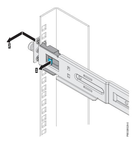
2. Remove the front bracket of the outer slide-rail from the rack by pulling the blue tab out **1** while you pull the end of the slide-rail away from the rack flange and toward the center of the rack **2**. Repeat step 1 and step 2 for the other outer slide-rail.
