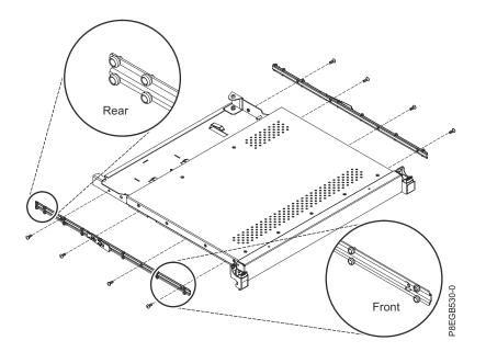
**12**. Go to Installing the console unit in the rack for instructions for reinstalling the console unit in the rack, and then install any other devices that you removed from the rack.
