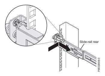
**c**. Extend the slide-rail and press the front slide-rail bracket towards the rack flange and then push it towards the rear of the rack until the locking bracket clicks into place behind the rack flange.
