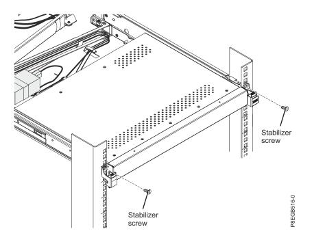
Before you move a rack with a console unit to another location, secure the front of the console unit to the rack with two M5 shipping screws that come in the bag of screws (see the illustration).
