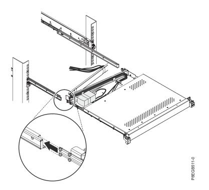
7. Press in both release latches 1; then, grasp both sides of the console unit and push it completely into the rack 2. There will be resistance initially as the inner and outer rails are aligned. Pull the console unit out halfway, and then push it back in to seat the console unit in the rails. Do this a few times until the console unit moves smoothly in the rails.
