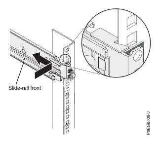
d. Repeat steps 4a to 4c to attach the other outer slide-rail.
