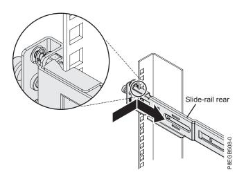
**c**. Extend the slide-rail and press the front slide-rail bracket toward the rack flange and then push it towards the rear of the rack until the locking bracket clicks into place behind the rack flange.
