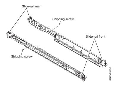
4. To attach the outer slide-rail to the rack, complete the following steps.
