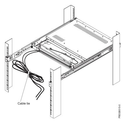
(Optional for all racks) To secure the slide-rails to the rack after installation, install an M5 flat-head stabilizer screw in the top hole on the front of each slide-rail.
