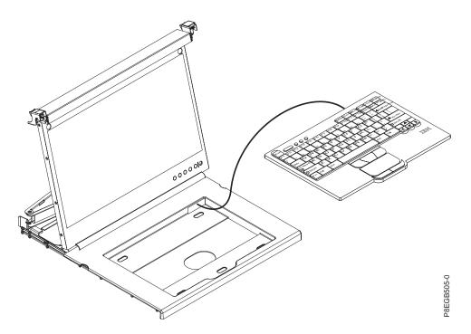
4. Peel the backing of the double-sided foam tape that is preinstalled on the front of the console tray.
