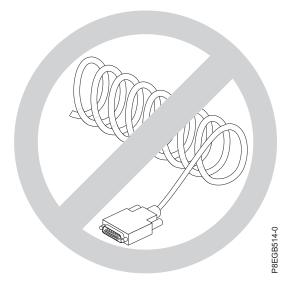
To minimize the electrical interference if you have excess video cable, arrange the cable in figure-eight loops, as shown in the following illustration. Secure the cable in the middle with a cable tie or strap.
