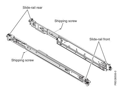
10. To attach the outer slide-rail to the rack, complete the following steps.
