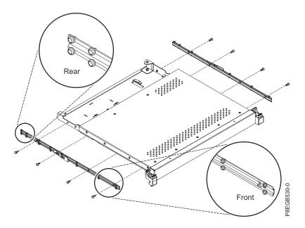
Carefully slide the console unit into the ball-bearing assemblies in the rails. Carefully slide the rollers on the console unit into the notch in the slide-rails as shown in the illustration.
