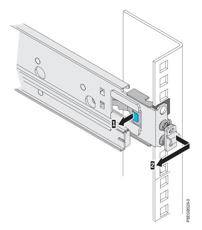
3. Remove the shipping screw from each new outer slide-rail.
