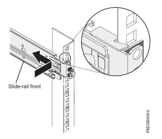
d. Repeat steps 5a to 5c to attach the other outer slide-rail.
