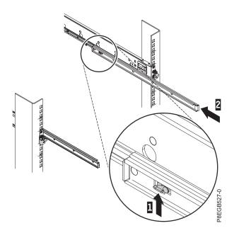
7. Remove the rear bracket of the outer slide-rail from the rack by pulling the blue tab out 1 while you move the end of the slide-rail away from the rack flange and toward the center of the rack 2.
