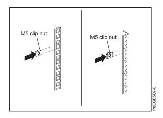
5. To attach the outer slide-rail to the rack, complete the following steps.
