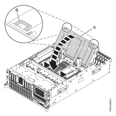
Figure 25. Closing the air baffle
