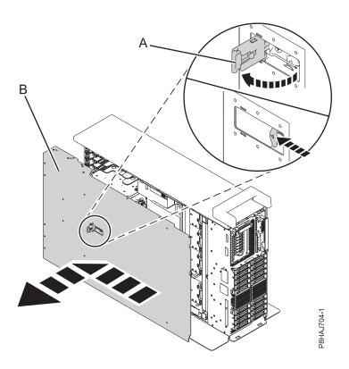
Figure 21. Removing the service access cover
