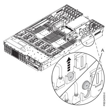
Figure 1. Removing the time-of-day battery
