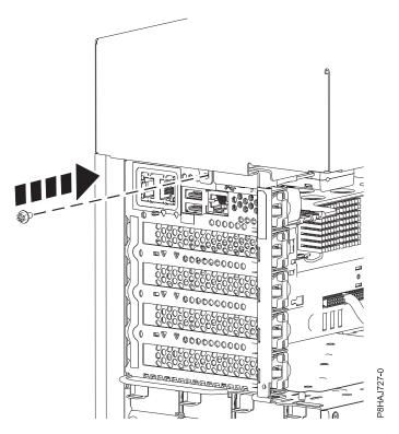
Figure 19. Installing the 8286-41A side cover screw
