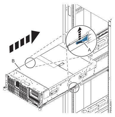
Figure 30. Placing the system into the operating position
