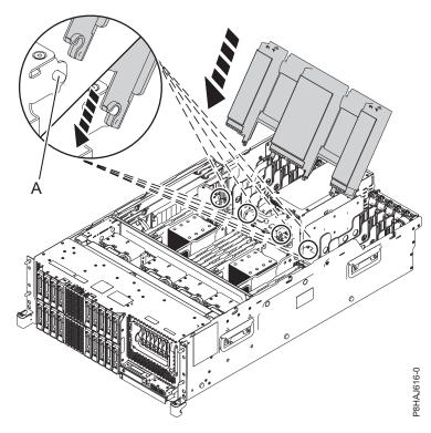
Figure 27. Replacing the air baffle
