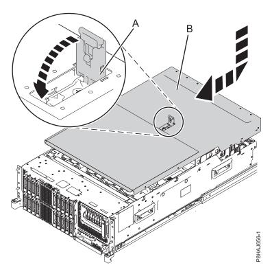
Figure 22. Installing the service access cover
