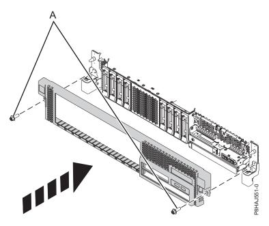
Figure 12. Installing the front cover
