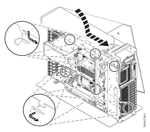
Figure 18. Installing the 8286-41A side cover
