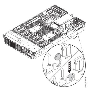
Figure 2. Inserting the time-of-day battery
