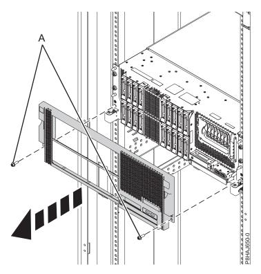
Figure 6. Removing the front cover
