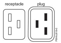
Figure 32. Connectors for the 8408-44E system
