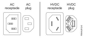
Figure 31. AC and HVDC connectors
