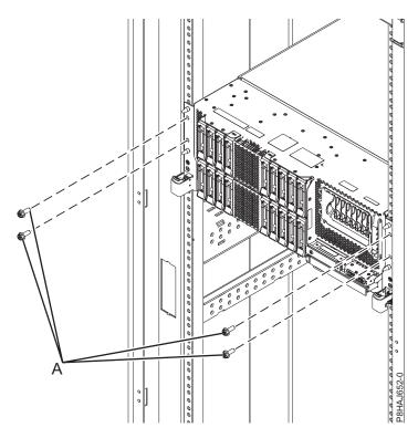
Figure 28. Removing the front screws
