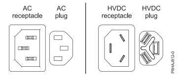
Figure 37. AC and HVDC connectors
