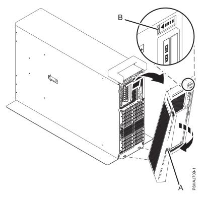
Figure 7. Removing the front cover
