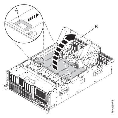
Figure 24. Opening the air baffle
