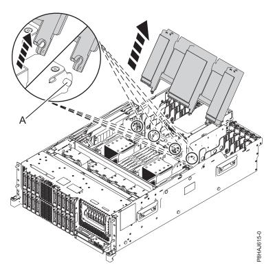
Figure 26. Removing the air baffle
