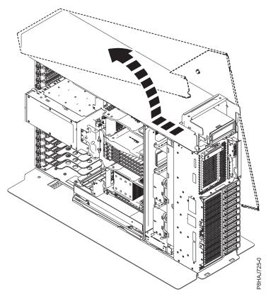
Figure 11. Removing the 8286-41A side cover
