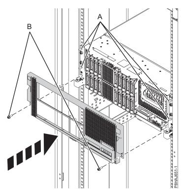
Figure 13. Installing the front cover
