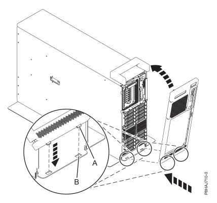
Figure 14. Installing the front cover
