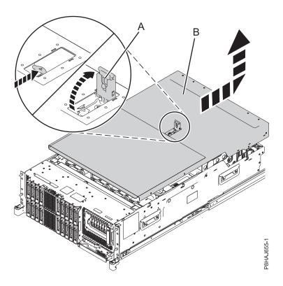
Figure 20. Removing the service access cover
