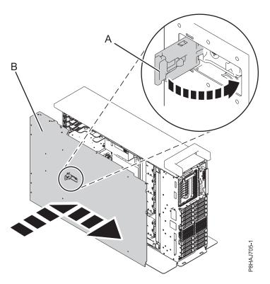
Figure 23. Installing the service access cover
