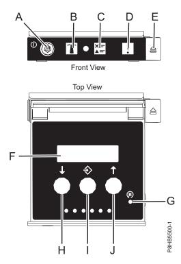
Figure 3. Control panel LEDs
