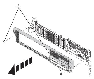
Figure 5. Removing the front cover
