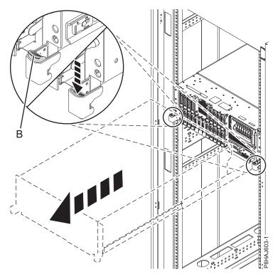
Figure 29. Releasing the side latches
