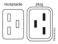
Figure 38. Connectors for the 8408-44E system
