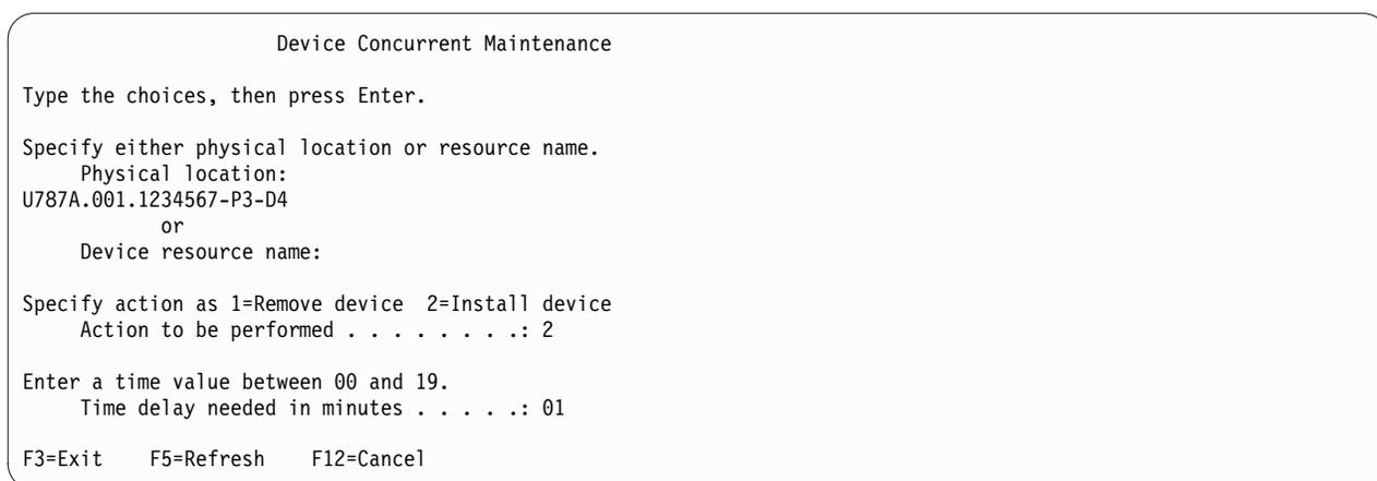
Figura 21. Exemplo Device Concurrent Maintenance display
