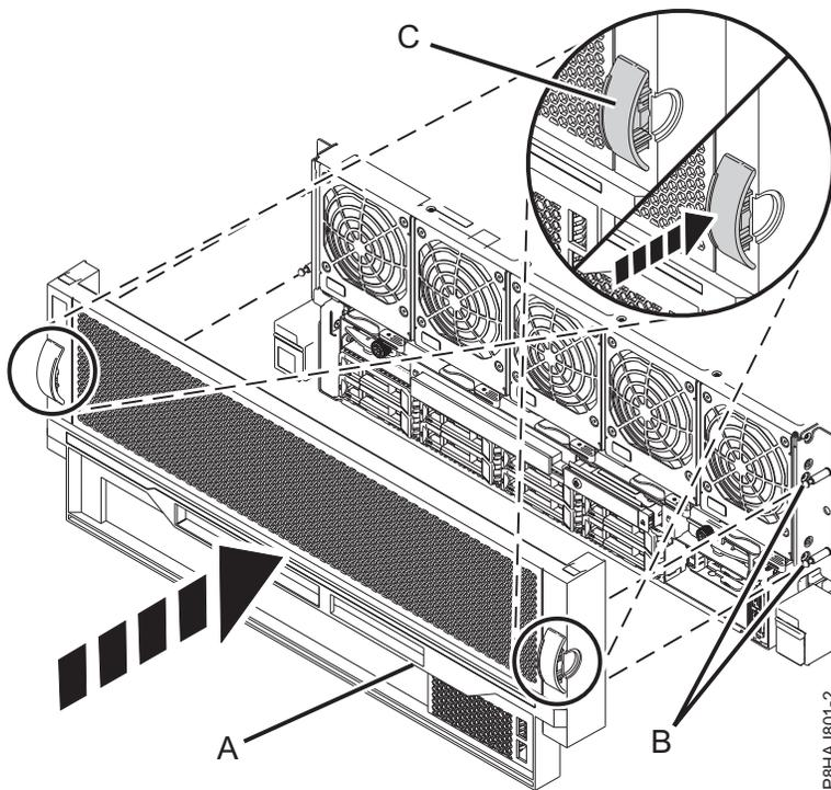
Figura 38. Instalando a Tampa Frontal
