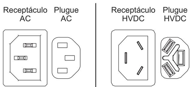
Figura 31. Conectores AC e HVDC
