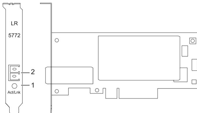
Figura 33. Adaptador PCI Express Ethernet-LR de 10 gigabits
