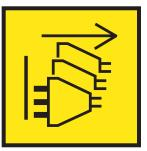
**DANGER:** Multiple power cords. The product might be equipped with multiple AC power cords or multiple DC power cables. To remove all hazardous voltages, disconnect all power cords and power cables. (L003)
