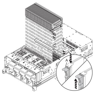
4. Push the CDIMM firmly into the slot until the tabs (A) lock.
