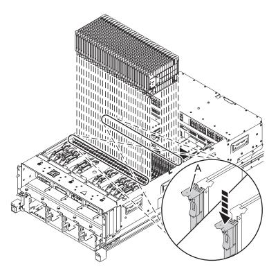
If you are not installing a new CDIMM, install the CDIMM filler if it is available.
