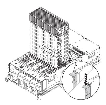
**Note:** CDIMMs are keyed to prevent a CDIMM from being installed incorrectly. Note the location of the key tab within the CDIMM connector before attempting to install the CDIMM.
