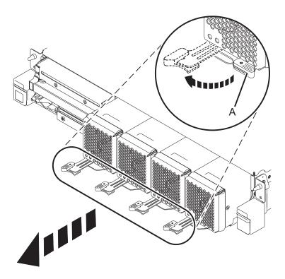
2. Pull the latch (A) to left to unlock the fan from its slot.
