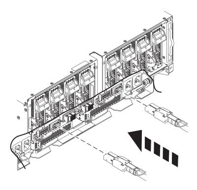
3. Lightly pull on the FSP cables from both attachment points to ensure it is locked into place. The cables should be firmly attached to the system.
