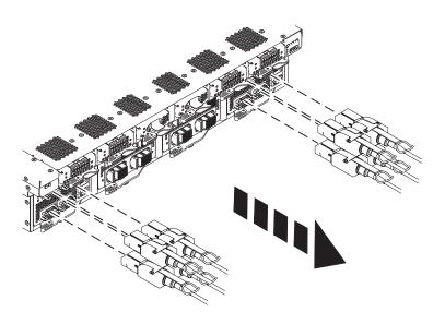
2. Unplug the other end of the FSP cable **being serviced** from the system node using the pull tab attached to the connector.
