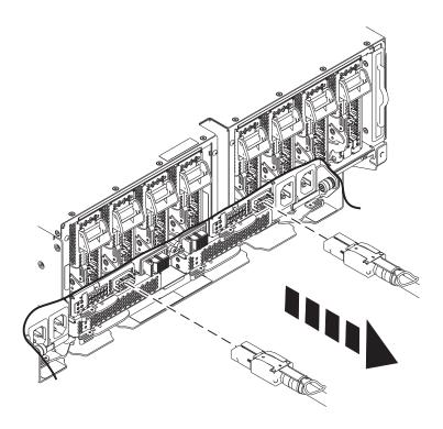
3. Loosen the hook-and-loop fastener securing the cable to the rack.
