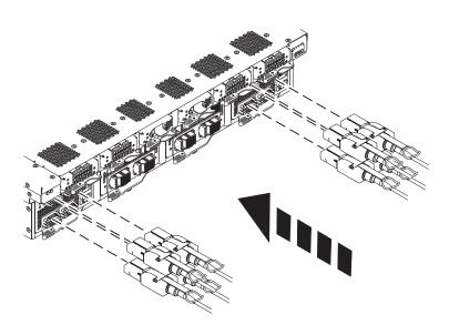
2. Plug the other end of the FSP cable into the system node by inserting the cable into the connector until it locks into place.
