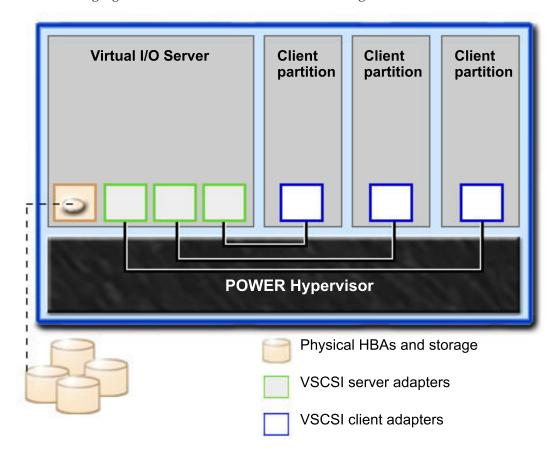
The following figure shows a standard virtual SCSI configuration.
