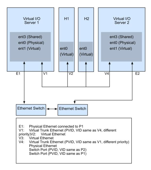
In this configuration, the default adapter of the Shared Ethernet Adapter that is illustrated as V1 in the figure, is used as control channel to manage the control channel traffic. A reserved virtual LAN is used for the control channel traffic. Multiple Shared Ethernet Adapters are configured in a high availability mode without a dedicated control channel adapter, and are supported in this configuration.
