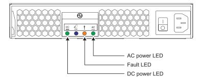
Figure 1. Rear view of power supply
